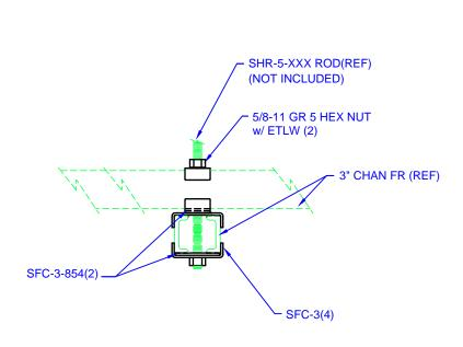
CONNECTION OF: 5/8 HANGER ROD TO 3" CHANNEL FRAMING AT CROSS-OVER
