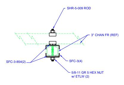
CONNECTION OF: 3"CHANNELS AT CROSS OVER (NOT A POINT OF SUPPORT)
