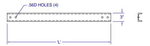
MATERIAL: 3"-4.1# STEEL CHANNEL (ASTM A-36)
