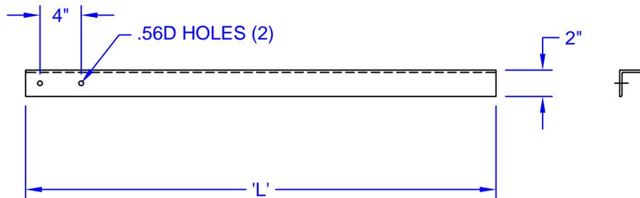
**MATERIAL: 2 x 2 x 3/16 STEEL ANGLE (ASTM A-36)**
